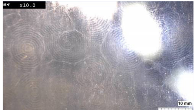
Thick tinning with typical circular structure
