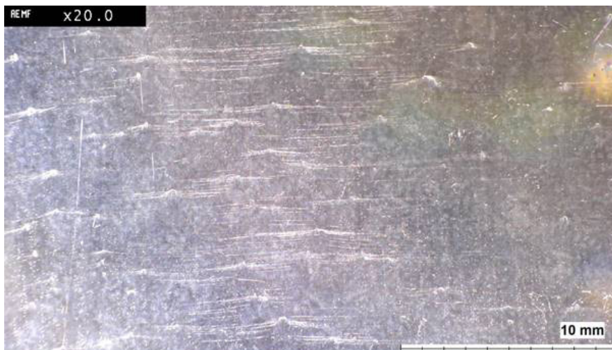
B14; 0.315mm; 1–3 \mu m tin layer thickness; SnPUR (blow-off direction vertical)
