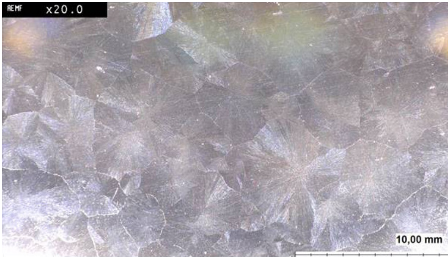
K81; 0.2mm; 1–3 \mu m tin layer thickness; SnTOP
