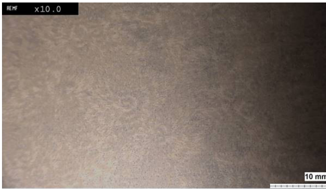
K65; 0.32mm; 1–2 \mu m tin layer thickness; SnTEM
