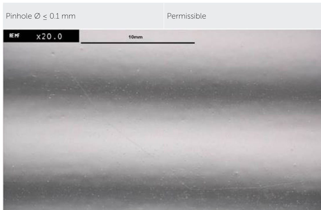
CuNiSi, C19010; 0.32mm material thickness, 3–6µm Sn
