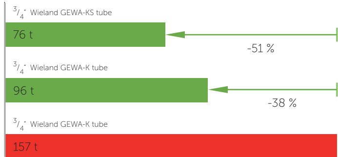
Capacity: 61 MW; TEMA type: NXN, 1-pass; shell Ø = 2,280 mm; number of tubes: 6467; propane (shell side):  $T_{sat}$  = 36 °C; cooling water (tube side):  $T_{inlet/outlet}$  = 22.0/31.2 °C
